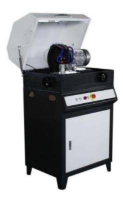
The EI-CM65 Metallographic Cutting Machine is a precision-engineered instrument designed for the efficient and precise interception of metallographic samples. It is engineered to prepare high-quality specimens without altering the material's microstructure, making it an indispensable tool for metallurgical education, failure analysis, and quality control across demanding industries such as automotive, aerospace, and mining.
